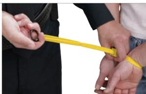
**Scarab Cutters** remove restraints with compound leverage.
